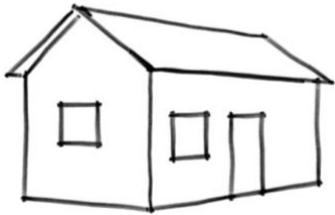
Twin roof creates two gables vulnerably exposed to strong winds.
