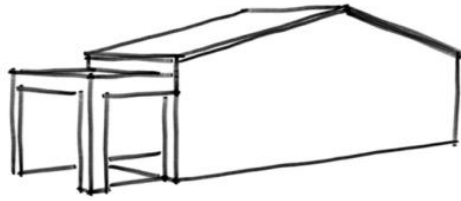
Large gable walls exposed to strong winds.
